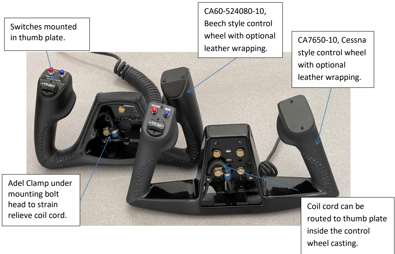
Figure 1: Front view of Beech and Cessna style control wheels mounted to adapters. Switches have been mounted in both wheels as typically done when installing Garmin GFC 500/600 auto pilots. The control wheels have provision to have the coil cord exit through the bottom of the wheel or through the back into the control column as needed. In both cases, the cable should be strain relieved. Face plates have been removed for clarity.
